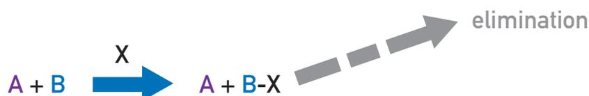
Undesired material B is eliminated via B-X precipitate, A remains unchanged
